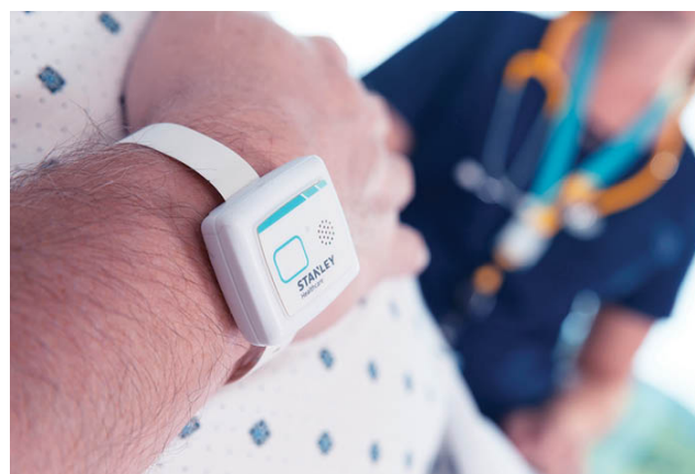
Figure 10: Real-time location system integrated to the patient's identification band
